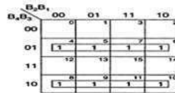
G_3 = B_4 \oplus B_3 K-map for G_3
